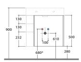
For the horizontal positioning of the hydraulic connections, consult the technical sheet of the selected sink
