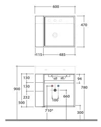
For the horizontal positioning of the hydraulic connections, consult the technical sheet of the selected sink
